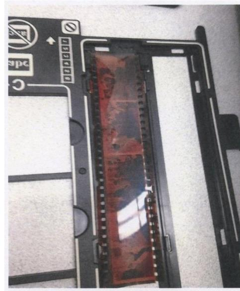
You will then line up the letter **"A"** on the attachment with the **"A"** on the scanner. Make sure if you are using Home Mode (recommended) to switch the document type to negative film (or whatever film type you have). Then select where you'd like to save it and hit scan.
