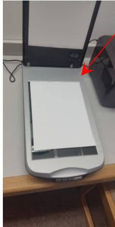
2. Once the scanner is closed, press the scan button when you are ready to scan and your scan menu will open up.
